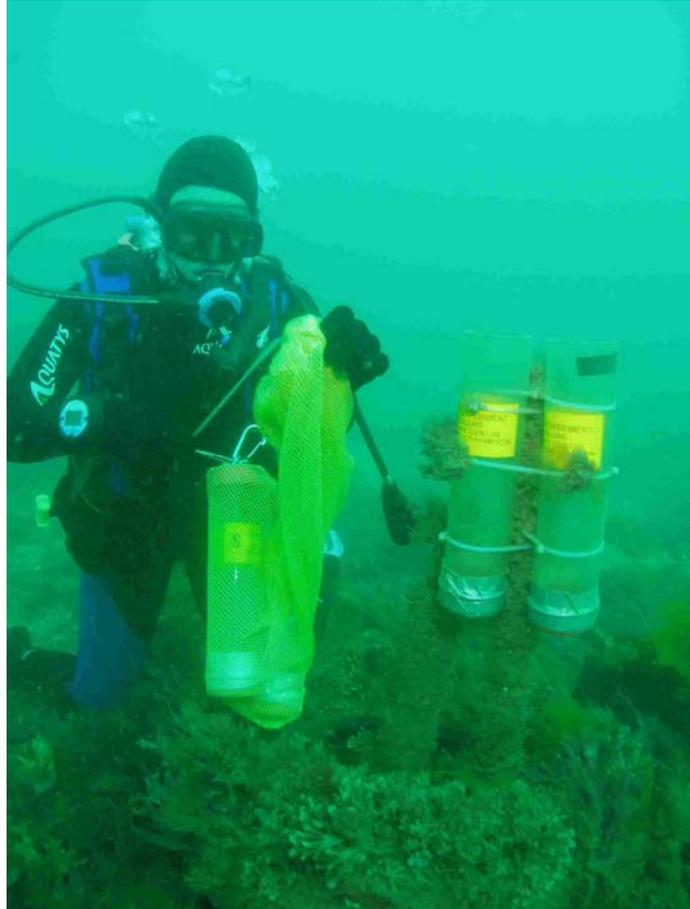
**Figure 2. Diver preparing to replace sediment traps on the Artificial Reef, Poole Bay**
