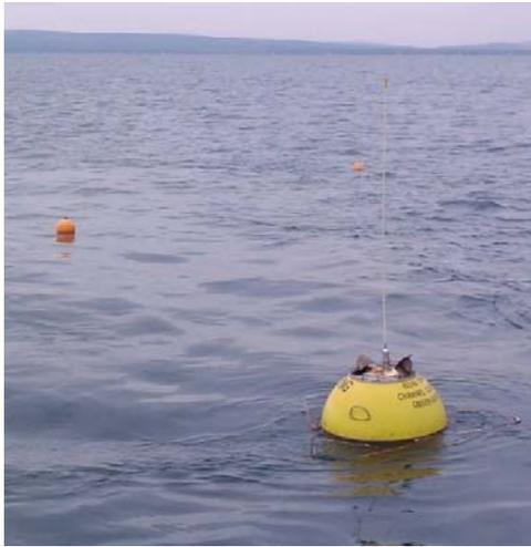
**Figure 15:** Datawell Directional Waverider buoy off Boscombe (Fugro EMU Limited)
